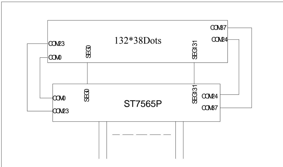
Figure 1. Block diagram
