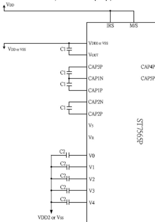
(2) When the voltage regulator internal resistor is not used.
