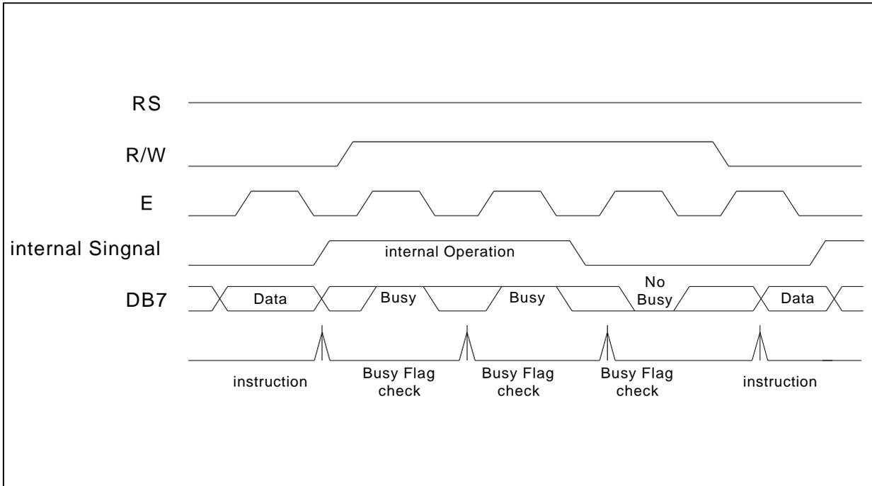
Example of 8-bit bus mode timing diagram
